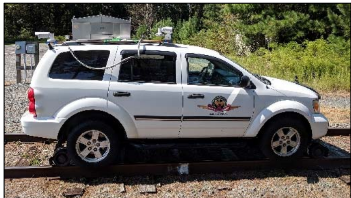
Figure 4 shows the thermal camera mounted to the rail maintenance truck.
